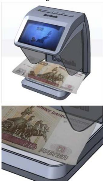
4. To activate special element "M" visualization press the
