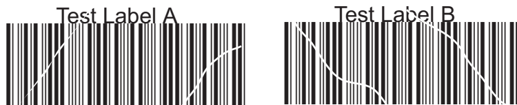
Low Quality Printouts Caused by Ribbon Wrinkling
